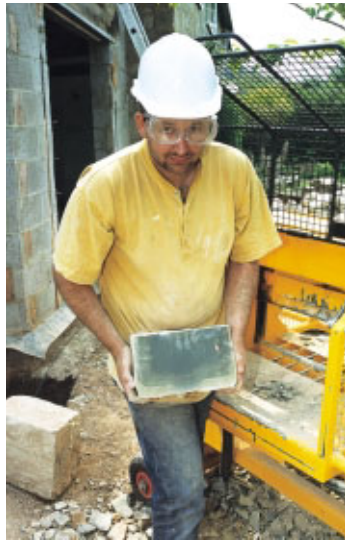
The productive Split-master soon turns unusable stone into desirable building material.
