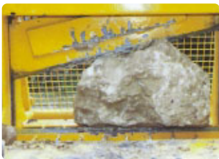
STEP 2 The Snell-split master angles its blade to the shape of the stone
